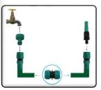
Designed to join hosepipes together.
